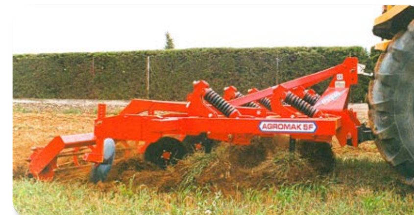
Tine protected with NO-STOP double spring for stony soils with stucks
