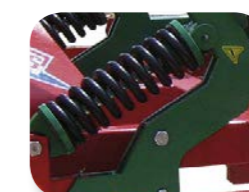
Tine protected with NO-STOP double spring for stony soils with stucks
