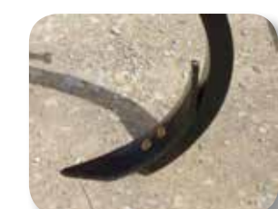
Two sided share made of boron steel
