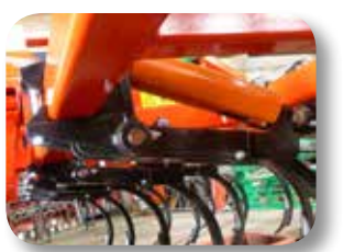
Reinforced frame with structural tubing
